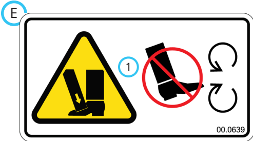
1. Pinching or crushing hazard - foot. Stay away from moving parts.
