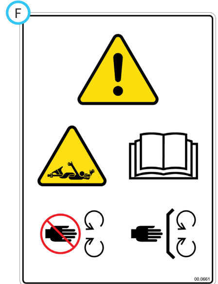
Danger - Rotating drive shaft. Stay away from moving parts. Do not operate with the drive shaft guards removed.
