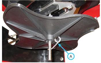
2. Slide the spinner blade or mulch basket down off the spinner shaft.
