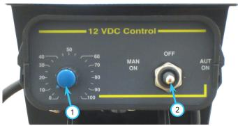
Power is sent to the motor by moving the switch to either MAN ON or AUT ON. Moving the switch to the MAN ON position disregards the speed control dial and sends full power to the motor. Moving the switch to AUT ON allows the motor speed to be controlled by the speed control dial setting.
