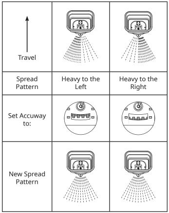
Moving the Accuway plate shifts the material on the spinner. Adjustment is very sensitive and should be done in small increments until the spread pattern is centered.
