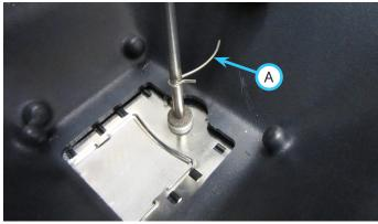
Use a pliers to grab the hook on the rotary agitator and pull the agitator back through the shaft to remove.
