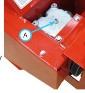
4. Reinstall the breather plug into the top port of the gearbox.
