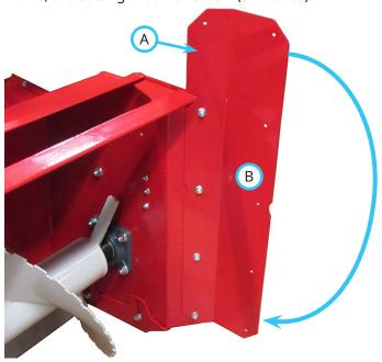
To switch from one cutting width to the other, rotate the vertical cutting edges 180 degrees. Do not switch the cutting edges to the opposite sides of the snow blower.
