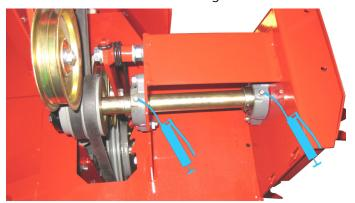
4. Lubricate the chute rotation chain.
