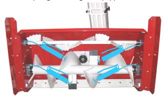
2. Grease the fan shaft bearings.
