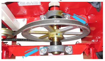
3. Grease the drive shaft bearings.
