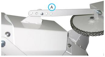
The discharge chute deflector adjustment link (A) controls the angle of the discharge chute deflector. The angle of the discharge chute deflector determines the distance that snow is thrown.
