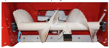
Reinstall the cutting edge onto the snow blower. When both sides of the cutting edge have been worn down, the cutting edge must be replaced.
