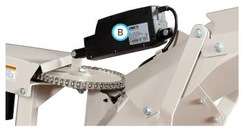
The optional actuator control (B) replaces the discharge chute deflector adjustment link on the snow blower. It couples with the 12 volt front switches\* on the power unit to control the angle of the discharge chute deflector from the operator's seat.
