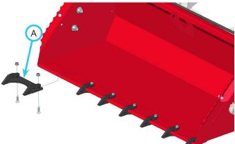
5. Secure each set of teeth to the power bucket using two 3/8 x 1-1/4 inch carriage bolts inserted up through the tooth and bucket. Secure with two flange nuts and torgue to 42 Nm (31 ft-lb).
