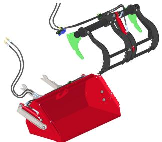
3. Install two 1/2 x 1-1/2 inch carriage bolts through both the right and left grapple frame brackets and the bucket sides and fasten with 1/2 inch nylon locking flange nuts. Torque to 102 Nm (75 ft-lb).
