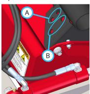
the right and left mounting brackets and secure with the nuts.
