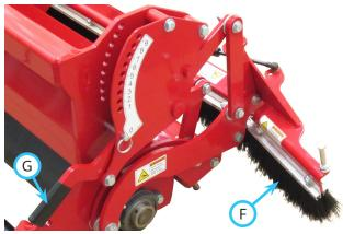
The groomer brush can be set to a fixed height by inserting a locking pin through the desired hole in the selector plate and the slot in the brush adjustment lever (G). Removing the locking pin will allow the groomer brush to float freely.
