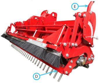
The spike bar can be set to a fixed height by inserting a locking pin through the desired hole in the selector plate and the slot in the spike bar adjustment lever (E). The spike bar can also be made more aggressive by lengthening the 3-point hitch top link or less aggressive by shortening the 3-point hitch top link.
