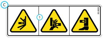
1. Pinching or crushing hazard.
