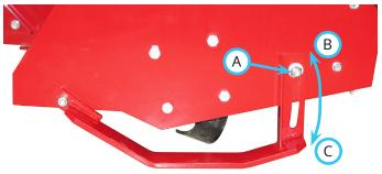
5. Check to make sure both the left and right skid shoes are set to the same position and tighten the adjustment bolts.
