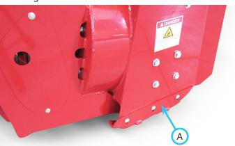
5. Retighten the skid shoe mounting nuts. Torque to 24 Nm (18 ft-lb).
