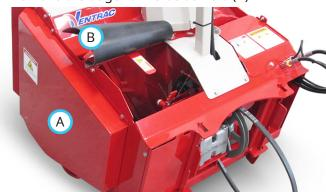
Flip open the belt adjustment cover belting (B).
