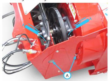
4. Lift up the belt adjustment cover belting and apply grease to the auger jack shaft bearings.
