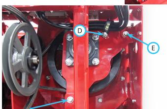
6. Remove the two bolts (E) that fasten the fan bearing mount plate to the snow blower frame.
