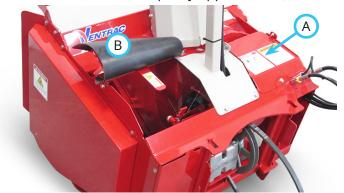
3. Flip open the belt adjustment cover belting (B).
