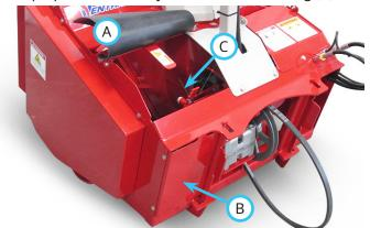
Remove the jack shaft drive shield (B).
