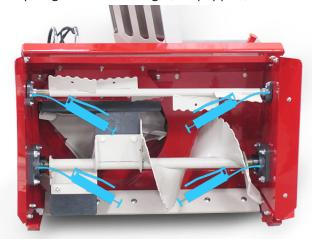
3. Apply grease to the fan shaft bearings. The grease fittings can be accessed through cutouts (A) in the right side panel and shield. The fan drive pulley upper shield can also be removed to provide access to the grease fittings.
