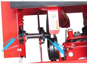
5. Apply chain oil or roller chain spray lube to the discharge chute rotation chain (B) and wipe up all drips and spills.
