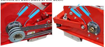
Grease the jack shaft bearings.
