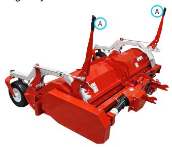
The height adjustment handles (A) are used to raise and lower the mower deck to the desired cutting height. The right and left adjustment handles must both be set to the same height position. The cutting height position decals list the adjustment handle positions and the corresponding cutting heights.
