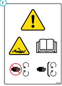
Danger - Rotating drive shaft. Stay away from moving parts. Do not operate with the drive shaft guards removed.
