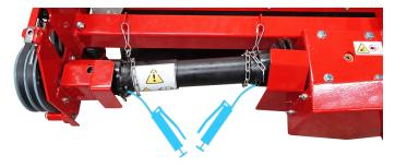
Grease the drive shaft universal joints.
