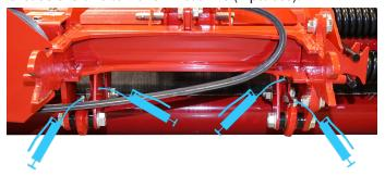
Grease the left rear roller bearing.
