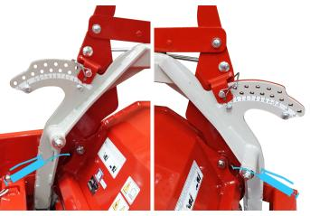
Set the height adjustment handles to position # 15. Grease the wheel axles and the wheel caster pivots.
