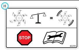
Missing, damaged, unbalanced, or excessively worn blades can affect the rotor balance. Do not operate in an unbalanced state. An unbalanced rotor will cause excessive vibration during operation. If the machine is operated in an unbalanced state, structural failure of frames and other components will result.
