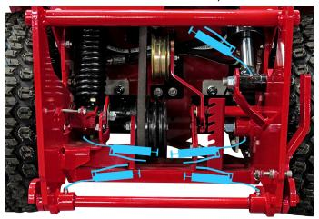
Remove the left engine shield and grease the lift cylinder upper end.
