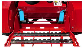
Lubricate the spherical rod ends on the valve control links.
