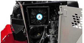
2. Remove the operator cushion to access the back of the cooler and use low pressure air to blow back through the oil cooler to remove accumulated dust or debris from the oil cooler fins.
