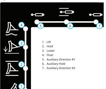
The hydraulic control lever controls the lift of the machine's front hitch and the auxiliary hydraulic circuit.
