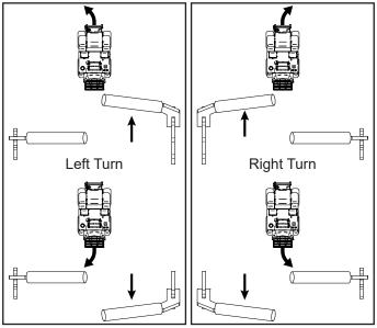
The greater the stroke variance between the left and right drive control levers, the sharper the machine will turn.
