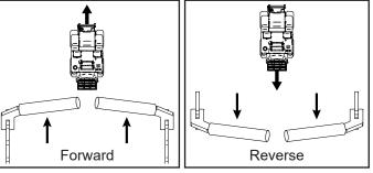
Pull the drive control levers backward to make the machine move in the reverse direction. Changing the amount the drive control levers are moved instantly changes the ground speed of the machine. Moving the drive control levers one half stroke will result in approximately one half of the maximum ground speed. Moving the levers to the end of the stroke will result in maximum ground speed.
