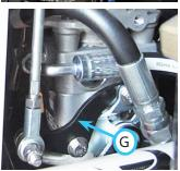
16. Push the right drive control handle forward until the tip of the drive handle just contacts the front control grab handle.
