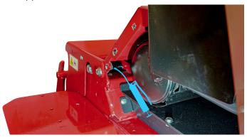
Lubricate the operator platform pivots.
