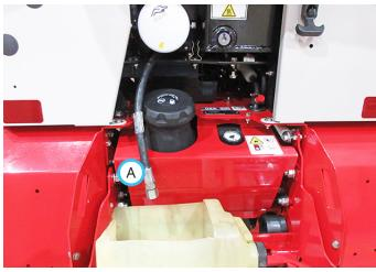
7. Remove the drain cap from the drain hose and drain the engine oil into the pan while the oil is warm.
