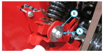
2. Check to see if the bolt is centered in the weight transfer slot as shown. If the bolt is not centered in the slot, the spring assembly length must be adjusted.
