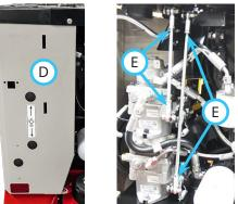
10. Loosen the jam nuts (E) from the rod ends on the pump link rod requiring adjustment and turn the rod to adjust the neutral lock plate. Lengthen the pump link rod to raise the neutral lock plate and shorten the rod to lower the neutral lock plate. The pump link rod will turn easily when tension is released and the bearings are not making contact with the neutral lock plates.
