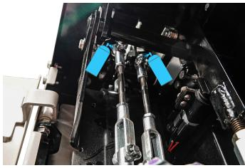
Lubricate the spherical rod ends on the pump control links.
