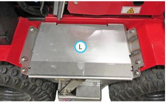
23. Install the controller and bracket onto the dash plate using two  $1/4 \times 3/4$  inch bolts (M), washers, and flange nuts. Insert the grommet on the power cord into the notch in the dash plate.
