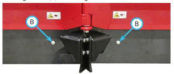
13. Install the new main cutting edges onto the V-blade. Torque the nuts to 42 N·m (31 ft-lb).
