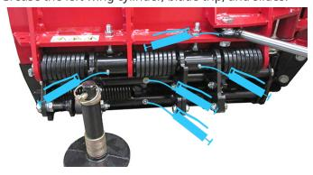
Grease the right wing cylinder, blade trip, and slides.
