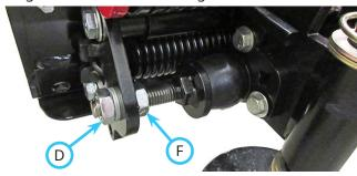
16. Torque the nuts (D) on the blade bumper stops to 205 N⋅m (151 ft-lbs).
