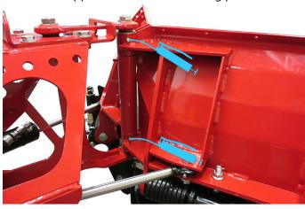
Adjust the blade wings to the swept back position and detach the V-blade from the power unit. Grease the wing blade cylinder ends.
