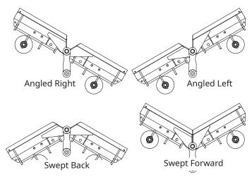
The blade wings can be angled independently from 30 degrees forward to 30 degrees backward. Angle the blade wings to the right or left to push snow to that side. Sweep the blade wings back to push snow to both sides. Sweep the blade wings forward to clear areas without the need for repeated cleanup passes.
