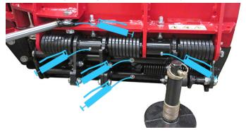
Grease the upper and lower blade wing pivots.
