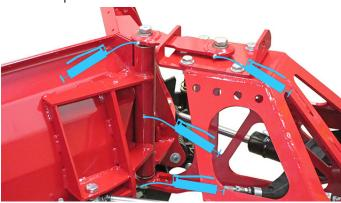
Grease the left wing cylinder, blade trip, and slides.
