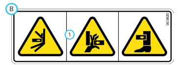
1. Pinching or crushing hazard.
