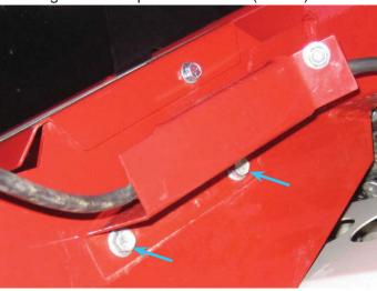
8. Run the wire harness inside the wire channel bracket. Place the clamp over the wire and insert the 1/4 x 5/8" flange bolt through the clamp flange and the wire channel bracket. Fasten with 1) 1/4" flat washer and 1/4" lock nut. Torque to 100 in-lbs (11 Nm).
