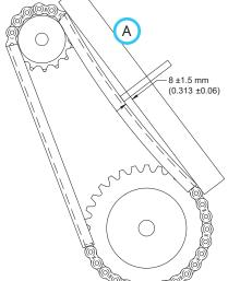
tension adjustment. If the chain tension is correct, reinstall the motor cover and torque the bolts to 11 Nm (100 in-lbs).
