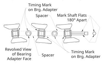
3. Install the required components in the sequence shown below. Double-check the timing mark locations and the spacer lengths (refer to the table) as each rotor is installed.
