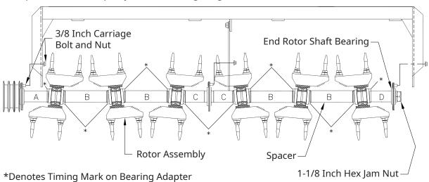
NOTES: 1. Each rotor assembly has the timing marks phased 180° apart on opposite sides.
