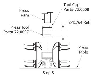
3. Press the used bearing and adapter assembly out of the rotor.
