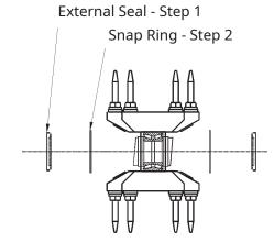
2. Remove the snap rings on both sides of the rotor.
