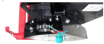
Optional Seeder - Oil the four rotor bearings. NOTE: to oil the seeder rotor bearings, place 3 - 4 drops of low viscosity oil between the rotor ends and the rotor bearings. The bearings are oil impregnated and will replenish themselves to their absorption capacity. Do not over-oil the bearings.
