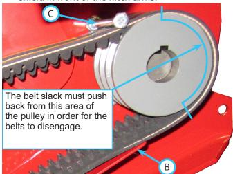
NOTE: the belt retainer bolt (C) and the bottom of the belt retainer shield (B) must keep the belt from moving very far away from the top or bot-
