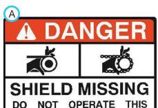
DO NOT OPERATE THIS MACHINE UNLESS ALL SHIELDS ARE IN PLACE. MOVING PARTS CAN CAUSE SERIOUS INJURY OR DEATH.
