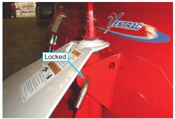
The unlocked position helps prevent sudden stops caused when contact is made with sidewalk joints, rocks, or other immovable objects. The unlocked position should always be used for snow removal. The pin can be installed in the outer hole to lock the blade trip mechanism. This position should only be used for digging or scraping at very slow speeds.
