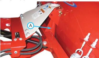
If the center pivot post leans forward, when the blade is angled to the left or right the leading edge of the blade will contact the ground while the trailing edge is still in the air. If the center pivot post leans backward, when the blade is angled to the left or right the trailing edge of the blade will contact the ground while the leading edge is still in the air.
