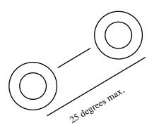
Keep engine oil level near full mark when operating on slopes.
