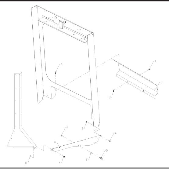
To install the left fender panel (C)(p.13), you will need to drill holes in the tractor fender. To locate the holes, bolt the two holes in the rear flange of the panel to the matching holes in the left post. After securing the rear of the fender panel, move the front of the panel into proper position and mark holes. See pictures and illustration below.
