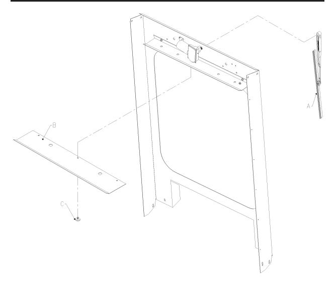
Install the electrical access cover (B) using 3)  $1/4 \times 1-1/4$  black knobs ©). Fasten to the u-bolts on the switch panel. Refer to illustration above and picture below.
