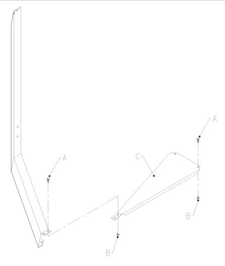
Remove the fender panel. Remove tractor tire while drilling holes and to access bolts when installing fender panel. Drill 2) 9/32 holes in the tractor fender. Bolt the fender panel into place using 4) 1/4 x 1/2 flange bolts (A) with 1/4 flange nuts (B). Install these four bolts from the inside. Reinstall tractor tire. Refer to pictures and illustration.
