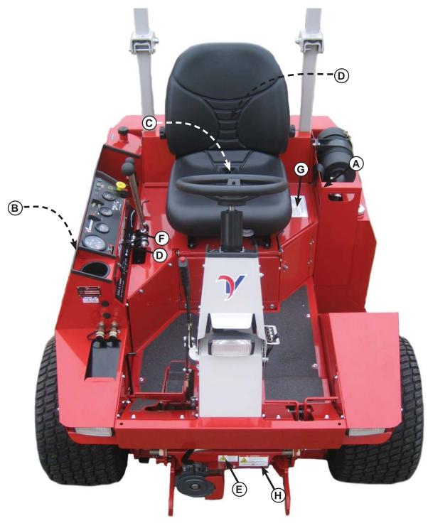
Note: Ref B located inside of shield and to the right of the battery. Ref C located in engine compartment on Radiator Shroud. Ref D located on inner crossmemeber of Rear Hood Screen.
