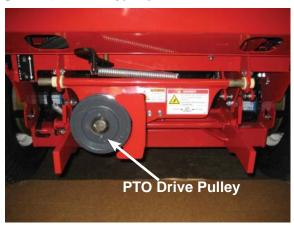
If the attachment requires a drive belt, then release the tension from the tractor drive PTO and install belt around the drive pulley at the location shown in the figure above. When belt is in place around the drive pulley, move the machine's PTO belt tensioner to the right to tighten the belt.
