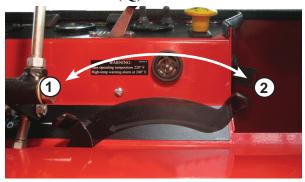
1 - S.D.L.A. control lever has a "spring assist to neutral" action. When removing your hand from the S.D.L.A. control lever it will automatically return to neutral. This position makes neutral easy to find and maintain. It is recommended that this position be used when learning the operation of the Ventrac, loading & unloading, attaching and removing attachments and whenever the operator is working in tight areas or unsure of the machines response to the task being performed.
