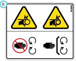
Fingers or hand entanglement. Stay away from moving parts. Keep all guards and shields in place.
