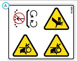
Shield missing - do not operate. Pinching/crushing hazard. Fingers or hand entanglement.
