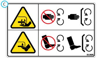
Cutting/dismemberment hazard of hand or foot, mower blade. Stay away from moving parts. Keep all guards and shields in place.
