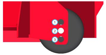
When the cutting height is set from 19 mm (3/4 inch) to 32 mm (1-1/4 inches), mount the anti-scalp rollers in position 1.
