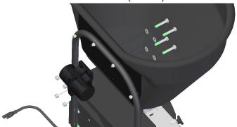
10. Remove the jam nut from the toggle switch. Install the toggle switch (A) into the hole in the control box mount bracket and fasten with the jam nut. Install the rub-
