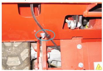
22. Use a plastic cable strap to fasten the cable to the front anchor plate, in order to keep the cable away from the left front tire and the disc brake.
