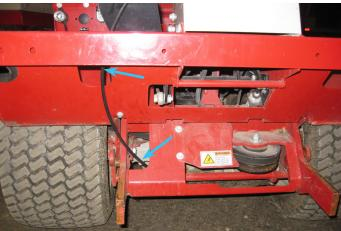
18. Route in front of the steering column and install the gate cable handle onto the gate cable mount.
