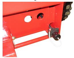
19. Route the battery/controller harness over to the right side of the rear frame following the main harness (G) behind the rear transaxle.
