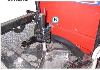
Install the agitator (C) onto the drive shaft. Apply blue thread lock to the set screw, align the set screw with the flat on the drive shaft, and tighten.
