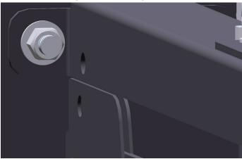
12. Fasten each side in place with a 3/8" x 3/4" ball pin.
