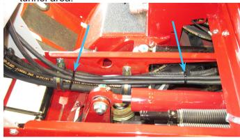
34. Use 2) zip ties to fasten the wire harnesses to the main wire harness in the center pivot area and in the rear frame next to the hydraulic oil tank.
