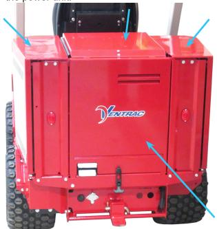
If the power unit is equipped with rear frame bottom covers (under the rear frame behind the transaxles), remove from the power unit.
