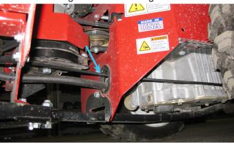
15. Route through the front frame cross member and forward along the left side of the front axle.
