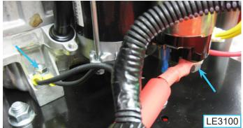
or use the supplied metric bolt and star washers to fasten to an unused threaded hole in the engine
