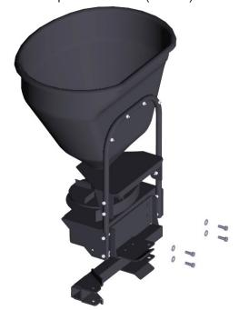
2. Install the spreader pivot hitch onto the tractor pivot hitch and align the holes in the spreader pivot plates with the hole in the tractor pivot tube. Place 2) 5/8" flat washers onto the 5/8" x 4-1/2"
