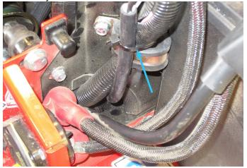
36. Use a zip tie to fasten the wire harnesses to the main wire harness in the rear frame behind the rear transaxle.
