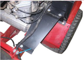
6. Use a zip tie to fasten the motor/controller wire harness to the exhaust heat shield with the end of the motor connector plug approximately 4" below the bottom of the rear frame.
