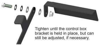
26. Fasten the controller bracket (J) to the control box mount bracket (K) using 2) #10-32 x 1/2" machine screws and #10-32 flange nuts.
