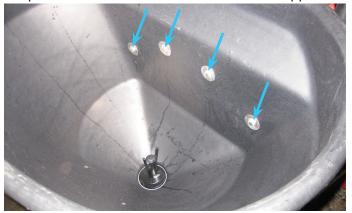
Remove the 4) bolts that fasten the hopper support plate (A) to the tube frame and remove the hopper support plate. The plate will not be reused.
