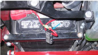
Plug the fused, split wire assembly into the positive lead at the battery and plug the original harness into the lead that splits from the new wire assembly. Use a zip tie to fasten the excess wire from the original harness to the new wire assembly and the air filter bracket.
