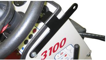
6. Place 2) disc springs onto a 3/8" x 1" bolt. Orient the disc springs so the peak of the coned disc is against the bolt head. Place a 3/8" flat washer onto the bolt and insert through the hole on the control box mount bracket as shown below. Place another 3/8" flat washer onto the bolt, install the control box bracket onto the bolt, and fasten with a 3/8" locking flange nut.
