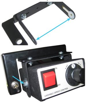
9. Install the control box mount bracket onto the control box bracket using 2) #10-32 x 1/2" machine screws and flange nuts.
