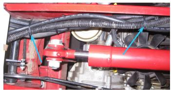
15. Route the wire harnesses through the center pivot area and fasten to the existing wire harness under the seat with a zip tie. Check to ensure that all linkages and moving parts do not interfere with the wires. Correct if necessary.
