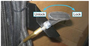
Pulling the cable out will open the gate and allow material to start flowing out of the hopper. Pushing in on the handle will then close the gate to stop the flow of material. It is suggested that the gate cable handle be locked by twisting it clockwise so the gate will not move from its selected position.
