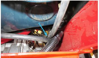
37. Use a zip tie to fasten the battery/controller harness to the main wire harness behind the rear transaxle on the left side of the rear frame.
