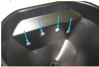
Place 1) 64.1686 vibrator mounting plate on the inside of the plastic hopper and the 2nd mounting plate on the outside of the plastic hopper.
