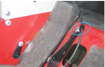
21. Install a supplied 1/4" x 3/4" bolt and clamp in the rear hole of the foot pedal pivot on the bottom side of the front frame. Place the gate cable in the clamp and tighten the bolt. Position the rear clamp in a manner that will not allow the cable to rub on the front hitch as the front hitch moves up and down.
