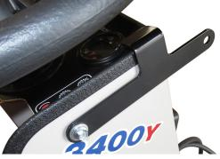
25. Place 2) disc springs onto a 3/8" x 1" bolt. Orient the disc springs so the peak of the coned disc is against the bolt head. Place a 3/8" flat washer onto the bolt and insert through the hole on the control box mount bracket as shown below. Place another 3/8" flat washer onto the bolt, install the control box bracket onto the bolt, and fasten with a 3/8" locking flange nut.
