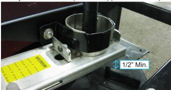
Move the hopper throat clamp in the gate mount slots until there is a minimum of 1/2" (12.7 mm) clearance between the spinner and the bottom of the gate assembly.
