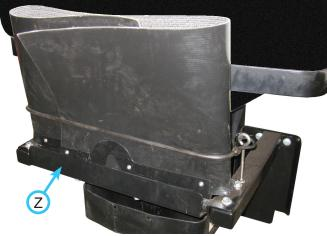
Secure by placing the bungee strap around the back of the drop curtain and hooking it onto the right eyebolt. If you prefer to completely remove the curtain from the spreader when not in use, it can be set up to be removed quickly. To set up for quick removal, unbolt the pivot tube clamps from the rear belting mount and reinstall the bolts, washers, and nuts to fasten the belting back onto the rear belting mount. Use the following procedure to remove the drop curtain for a wider spread pattern.
