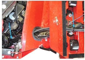
35. Use a zip tie to fasten the battery/controller harness to the main wire harness in front of the battery.
