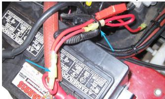
3. Install the negative wire assembly onto the engine ground bolt. Torque bolt to 210 in-lbs (24 Nm).
