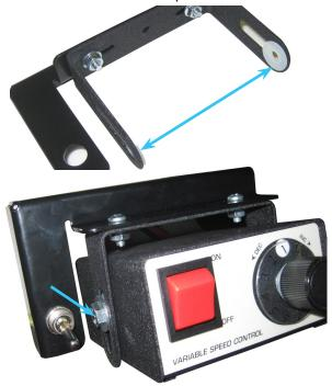
28. Install the control box mount bracket onto the control box bracket using 2) #10-32 x 1/2" machine screws and flange nuts.
