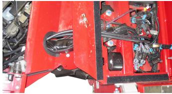
22. Follow the front wire harness through the tunnel area and up through the steering column, exiting the steering column at the head light mount.
