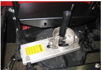
24. Place the plastic hopper throat into the gate assembly and temporarily install a cushioned metal clamp to both of the outer hopper mounting holes. Do not tighten as these will be removed again. Route the gate cable through the two clamps.
