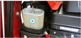
5. To loosen debris, gently tap the filter element on a hard surface. If the filter element is excessively dirty, replace it with a new air filter element.
