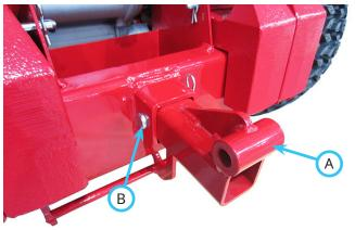
Align the RV tractor hitch (A) with the collection vacuum hitch (C) and back slowly into position. If the collection vacuum is not at the correct height, turn the storage stand handles (D) to raise or lower the collection vacuum to the correct height. NOTE: the power unit hitch height can be affected by the terrain, the tire pressure, and the attachment on the front of the power unit.
