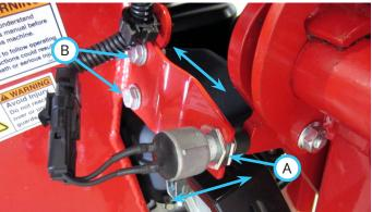
If the switch needs to be adjusted from side to side, loosen the bolts (B) that fasten the switch bracket to the fan housing and move the switch bracket until the switch is centered with the right bin lift arm. Torque the bolts to 24 Nm (210 in-lbs).
