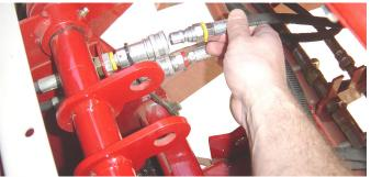
7. Connect the battery cable to the quick connect plug on the power unit.
