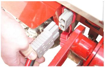
8. Rotate the docking station handle (K) to release the collection vacuum from the docking station.
