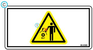
Cutting / dismemberment / entanglement hazard -Do not remove shields.
