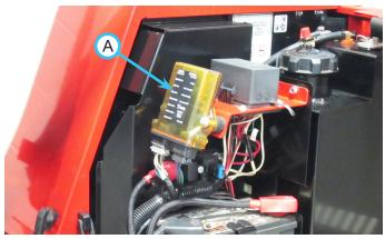
The Tractor Control Module (A) is a sealed computerized device designed to control the electronic safety related functions of this tractor. Both solid state and mechanical components are used to assure safe, reliable operation of this machine.
