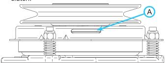
2. Place a .020" (.5 mm) feeler gauge in the slot between the armature and the rotor.
