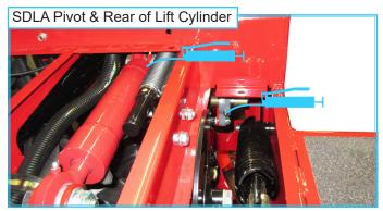
The rear grease fitting on the lift cylinder must be greased from below the cylinder by removing the weight transfer access cover and using a grease gun with a flexible hose.
