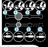
The SDLA(Speed, Direction, Lift, and Auxiliary) is the primary control for the power unit and consists of two levers. The primary SDLA control lever (L) controls the speed, direction of travel, and lift of the hitch arms. The secondary SDLA control lever (M) controls the auxiliary hydraulic circuit.
