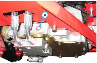
9. Clean the drain plug, reinstall into the front transaxle, and torque to 22 ft-lbs (30 Nm).
