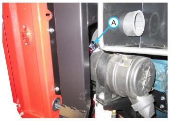
To check the air filter restriction gauge:
