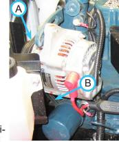
10 kgf). The belt deflection should measure 1/4 to 3/8 inches (7 to 9 mm). If the belt deflection is not within specifications, the belt tension must be adjusted.
