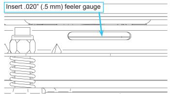
3. Tighten or loosen the clutch adjustment nut (B) as needed to achieve the .020" (.5 mm) air gap.
