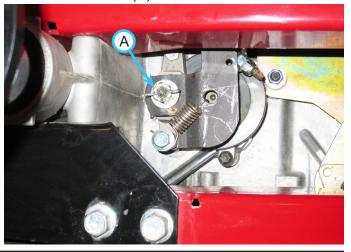
8. If the amount of force required to engage the selector lever into the park position was less than 15 pounds (7 kg), turn the castle nut tighter by one position. If the amount of force required to engage the selector lever into the park position was greater than 22 pounds (10 kg), loosen the castle nut by one position.
