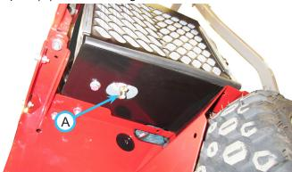
7. Turn the drain valve counterclockwise to open and drain the coolant into the drain pan.
