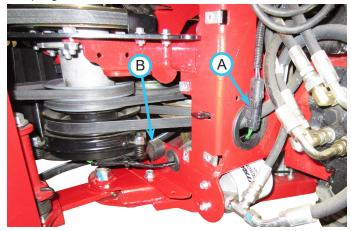
Remove the two rubber bumpers (B) from the front frame (one on each side of the PTO clutch).
