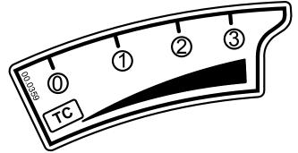
The weight transfer system transfers weight from the attachment to the front wheels of the power unit. Transferring weight from the attachment to the power unit increases the traction control, improves hillside maneuverability, aids in lifting the attachment, reduces steering effort, and lessens the attachment resistance when in contact with the ground.
