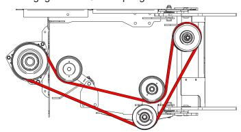
13. Check to ensure the belt is properly seated in the pulleys.
