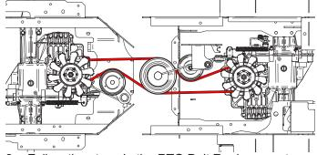
9. Follow the steps in the PTO Belt Replacement section to install the PTO belt onto the PTO clutch.
