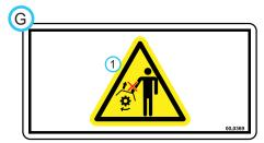
Cutting / dismemberment / entanglement hazard - Do not remove shields. Stay away from moving parts.
