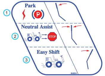
1 - In this position, the park brake is applied. The lever must be in this position for starting. When leaving the seat with the engine running, the lever must be in this position or the power unit will automatically shut off. The foot pedal control and the S.D.L.A. control lever are locked while in this position.
