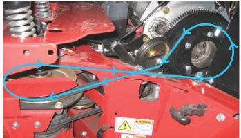
8. When installing a new drive belt, verify idler pulley position as indicated in the Drive Belt Adjustment section of the manual.
