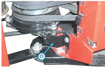
7. Release the tension from the PTO belt by unlatching the two extension arms of the torsion spring that is a part of the PTO idler pulley assembly. This is located behind the right front tire (see figure below).
