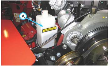
6. Visually inspect to see that the level of hydraulic oil is centered between the low and full marks of the tank. Note: use a flashlight to inspect level if necessary. 7. If hydraulic oil level is low, remove the cap from the hydraulic tank (A) and add HydroTorq XL synthetic hydraulic oil until level is centered between the low and full marks of the tank.
