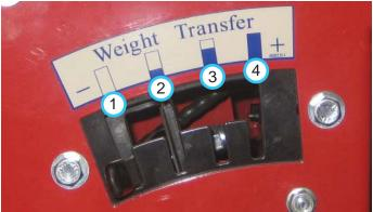
The weight transfer system allows the operator to select the amount of weight transferred from the front mounted attachment to the front drive wheels of the power unit. Transferring weight from the attachment to the power unit improves traction and hillside stability, aids in lifting, reduces steering effort, and lessens the attachment resistance when in contact with the ground. Note: The weight transfer system is only active while the primary S.D.L.A. is in the float position.
