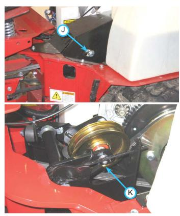
If position of the bolt and indicator bracket are not in-line, then the position of the engine cradle will need adjusted. To adjust the engine cradle position, loosen the four engine cradle bolts as shown at the locations shown below.
