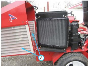
Clean all debris from outer screens (A) around the hood with a brush, compressed air, or water. NOTE: be sure to blow or spray from the inside out.
