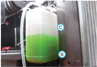
NOTE: when cold, the level should be between Low (B) and Full (C) marks on the tank.
