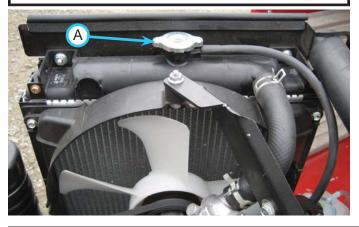
slightly and continue to turn counterclockwise and remove cap from radiator. Check that the coolant level is up to the bottom of the filler neck.
