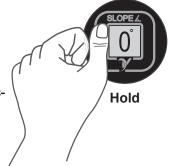
Starting below the sensor area, swipe your thumb up across the sensor to scroll through options such as audible and visual alert set-points or display screen options.
