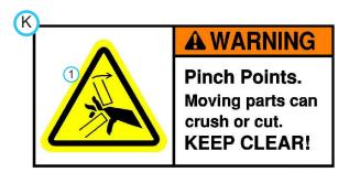
$\hbox{1. Cutting/crushing hazard - Stay away from moving parts.}\\$
