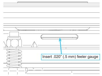
3. Tighten or loosen the clutch adjustment nut (B) as needed to achieve the .020" (.5 mm) air gap.
