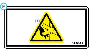
Cutting/dismemberment/entanglement hazard - Stay away from moving parts.
