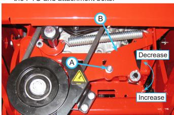
6. Tighten the adjustment bolt securely. Torque to 31 ft-lbs (42 Nm).
