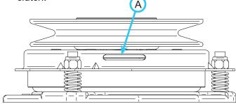
2. Place a .020" (.5 mm) feeler gauge in the slot between the armature and the rotor.
