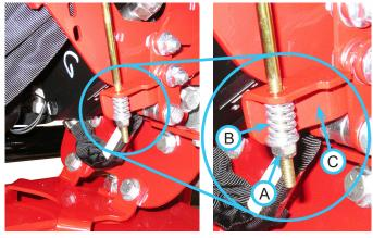
6. After the required amount of force to engage the brake lever is achieved, disengage the parking brake and move the SDLA lever forward as far as it will go. While moving the SDLA lever forward, observe the compression spring (B) and brake engagement tab (C) on the brake linkage. The compression spring on the brake linkage rod should not cause the brake engagement tab to be lifted up more than .03" (.8 mm). If the
