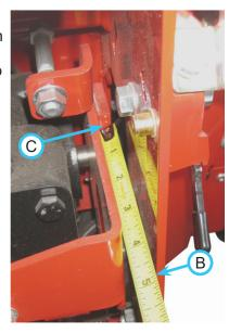
between the front frame and the pump arm. This measurement should be a minimum of 1/32" (.8 mm) less and a maximum of 1/16" (1.6 mm) less than the measurement taken in step 9 (ex. if measurement in step 9 was 4" (101.6 mm), the measurement when the light goes out must be between 3-31/32" (100.8 mm) and 3-15/16" (100 mm)).
