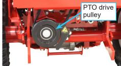
drive pulley at the location shown above. When the belt is in place around the drive pulley, push the PTO belt tensioner rod in to engage and tighten the belt.
