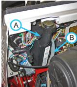
7. If the hydraulic oil level is below the low mark on the decal, add HydroTorq XL synthetic hydraulic oil until the proper level is reached.
