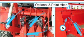
The front grease fitting on the 3 point cylinder can be greased through an access hole (A) in the right foot platform panel.
