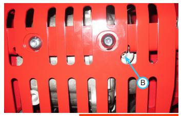
3. Remove the drain plug (B) from the rear transaxle and allow the hydraulic oil to drain from the system. Remove the oil fill plug (C) from the rear transaxle to allow venting. NOTE: on some
