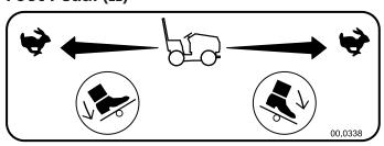
The foot pedal works in conjunction with the SDLA control lever and can be used to control the speed and direction of the power unit when the operator's hand is removed from the SDLA lever.
