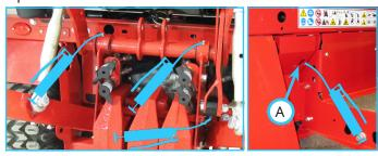
The front grease fitting on the 3 point cylinder can be greased through an access hole (A) in the right foot platform panel.
