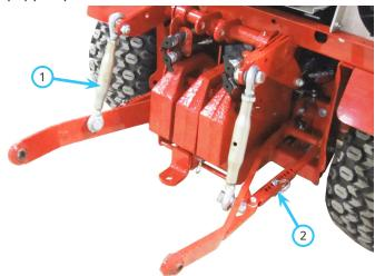
The optional 3 point hitch is equipped with adjustable lift links (1) to control the individual draw bars. The stabilizing links (2) can be allowed to swing freely or can be locked at a desired position.
