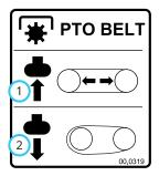
Pulling the PTO belt tensioner rod out (2) releases the belt tension, allowing the operator to remove or install the attachment drive belt.
