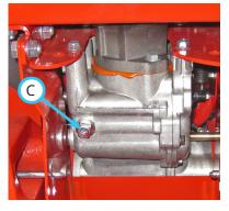
may be necessary to remove the rear transaxle skid plate to access the drain plug.
