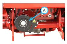
the belt is in place around the drive pulley, push the PTO belt tensioner rod in to engage and tighten the belt
