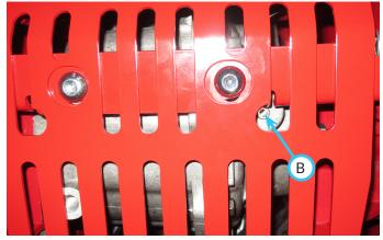
3. Remove the drain plug (B) from the rear transaxle and allow the hydraulic oil to drain. Remove the oil fill plug (C) from the rear transaxle to allow venting. NOTE: on some power units, it
