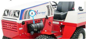
2. Release both latches (B) on the engine air filter assembly (A) and unhook the latches from the main filter housing.
