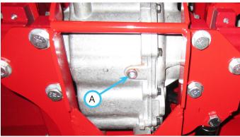
7. If the transaxle is equipped with a pipe plug, clean the drain plug and apply pipe sealant to the threads, making sure to leave the last two threads bare to prevent the thread sealant from contami-
