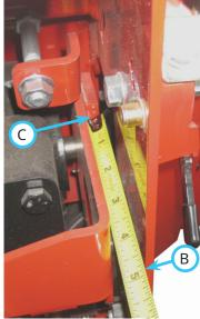
less than the measurement taken when the SDLA lever was at the neutral position. (e.g., if the original measurement was 101.6 mm (4 inches) the measurement when the neutral switch input light turns off must be between 100.8 mm (3-31/32 inch) and 100 mm (3-15/16 inch). NOTE: it is helpful to have an assistant to take the measurements.
