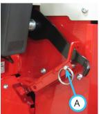
Ensure the shift lever is secured in the lock position at the end of the shift stroke. Reinstall the
