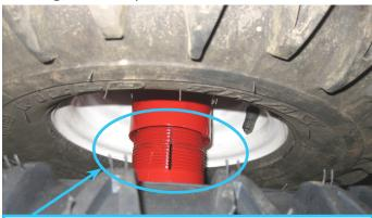
After tightening the outer dual wheel, there should be four or fewer threads visible on the outer dual wheel extension.
