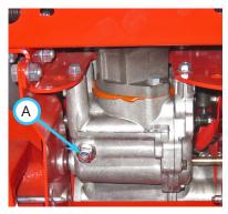
the bottom of the oil fill hole.
