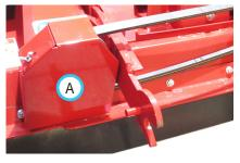
4. Reinstall the drive pulley shield.
