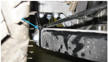
23. Place the gate assembly over the agitator and spinner drive shaft with the cable connection point on the left side.
