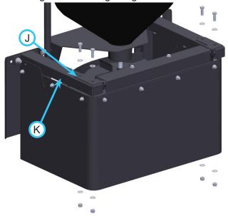
6. Tighten the 8) 5/16" bolts (L) that fasten the right and left drop curtain mounts to the hopper support tube, transmission mount plate, and hopper support plate. Torque to 135 in-lbs (15 Nm).
