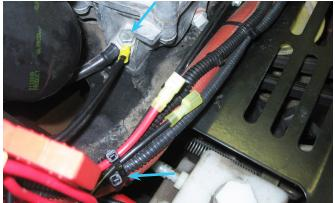
4. Use a zip tie to fasten both the positive and negative leads to the existing wire harness as shown above.
