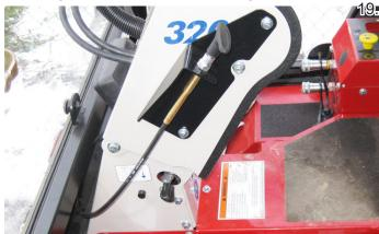
20. Remove the bolts that fasten the foot pedal pivot to the front frame. Install a supplied 1/4" x 3/4" bolt and clamp in the front hole of the foot pedal pivot on the top side of the front frame. Place the gate cable in the clamp and tighten the bolt.
