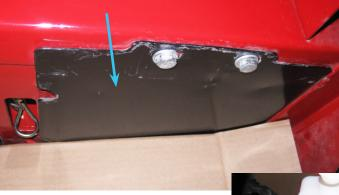
5. Route the motor/controller harness back along the power unit's rear wire harness, under the hydraulic oil reservoir, between the engine frame and the rear axle, and back up behind the engine.
