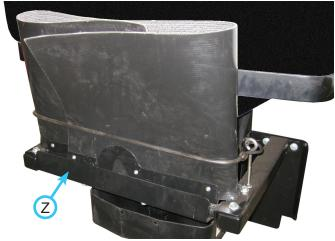
5. Secure by placing the bungee strap around the back of the drop curtain and hooking it onto the right eyebolt.
