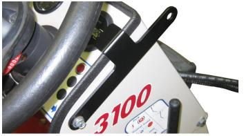
Place 2) disc springs onto a 3/8" x 1" bolt. Orient the disc springs so the peak of the coned disc is against the bolt head. Place a 3/8" flat washer onto the bolt and insert through the hole on the control box mount bracket as shown below. Place another 3/8" flat washer onto the bolt, install the control box bracket onto the bolt, and fasten with a 3/8" locking flange nut.
