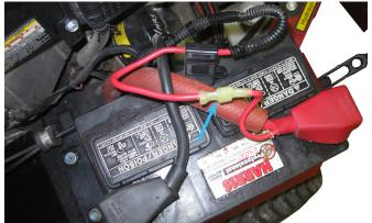
2. Plug the fused, split wire assembly into the positive lead at the battery and plug the original harness into the lead that splits from the new wire assembly. Use a zip tie to fasten the excess wire from the original harness to the new wire assembly.
