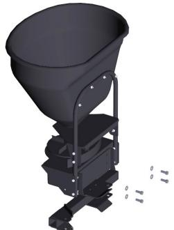
Install the spreader pivot hitch onto the tractor pivot hitch and align the holes in the spreader pivot plates with the hole in the tractor pivot tube. Place 2) 5/8" flat washers onto the 5/8" x 4-1/2"
