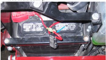
2. Plug the fused, split wire assembly into the positive lead at the battery and plug the original harness into the lead that splits from the new wire assembly. Use a zip tie to fasten the excess wire from the original harness to the new wire assembly and the air filter bracket.
