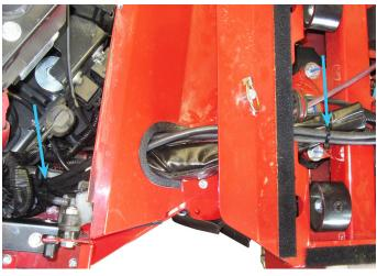
35. Use a zip tie to fasten the battery/controller harness to the main wire harness in front of the battery.
