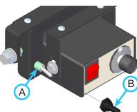
ber toggle switch boot (B) onto the toggle switch.
