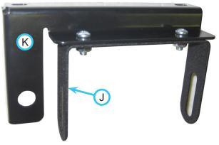
27. Place the nylon washers on the inside of the controller bracket and install onto the controller using the 1/4" bolts and flat washers. Tighten the bolts until the controller pivots with resistance.
