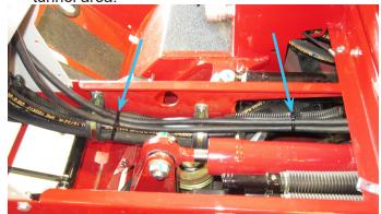
34. Use 2) zip ties to fasten the wire harnesses to the main wire harness in the center pivot area and in the rear frame next to the hydraulic oil tank.
