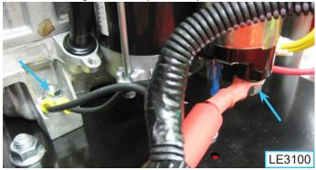
or use the supplied metric bolt and star washers to fasten to an unused threaded hole in the engine
