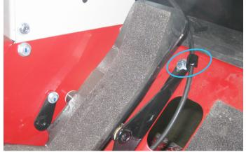
21. Install a supplied 1/4" x 3/4" bolt and clamp in the rear hole of the foot pedal pivot on the bottom side of the front frame. Place the gate cable in the clamp and tighten the bolt. Position the rear clamp in a manner that will not allow the cable to rub on the front hitch as the front hitch moves up and down.
