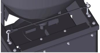
11. Rotate each side of the drop curtain up into place with one of the side curtain mounts on each side of the side belting hanger flange until the mounting holes are aligned.
