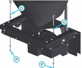
10. Fasten the clip on the supplied polymer bungee strap to the left eyebolt and hook the opposite end onto the right eyebolt.
