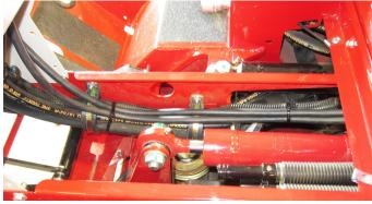
23. Place the steering column cover back onto the steering column using care not to pinch the wire harnesses. Do not fasten.
