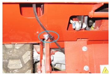
22. Use a plastic cable strap to fasten the cable to the front anchor plate, in order to keep the cable away from the left front tire and the disc brake.
