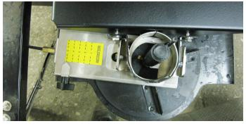
Drill a 3/8" (9 mm) hole in the belting and use a utility knife to cut a slice in the belting so the cable can pass through the curtain.
