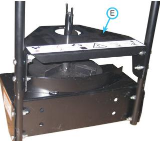
4. Insert the hopper throat into the hopper support plate and fasten the hopper to the hopper support tube using 4) 5/16" x 2" bolts, 5/16" x 1-1/2" fender washers, and 5/16" locknuts. Torque to 135 in-lbs (15 Nm).
