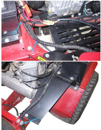
6. Use a zip tie to fasten the motor/controller wire harness to the exhaust heat shield with the end of the motor connector plug approximately 4" below the bottom of the rear frame.
