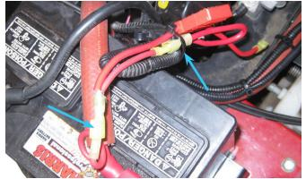
3. Install the negative wire assembly onto the engine ground bolt. Torque bolt to 210 in-lbs (24 Nm).
