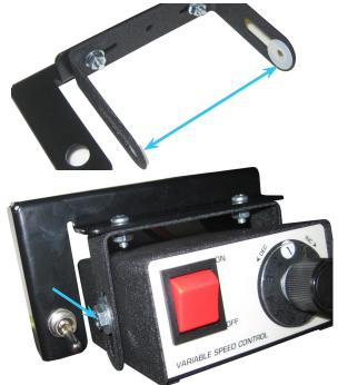
Install the control box mount bracket onto the control box bracket using 2) #10-32 x 1/2" machine screws and flange nuts.
