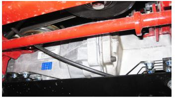
17. Route through the opening in the front hitch and up through the hole in the frame next to the foot pedal.
