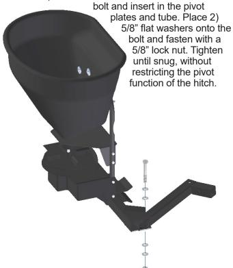
3. Pivot the spreader hitch until the pivot lock holes are aligned and fasten with a 5/8" x 3" hitch pin.
