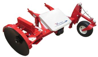
It is recommended when setting up the edger for bed shaping to rotate the disc assembly so the disc is behind the main frame receiver tube. To set up the edger for bed shaping:
