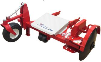
Refer to the Disc Position Setup section for instructions on rotating the disc to the front or rear of the receiver frame tube.
