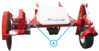
2. Insert the gauge wheel assembly into the right side of the frame receiver tube and secure with the ball pin.
