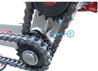
8. Tighten the locking nuts to secure the stop bolt.
