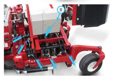
Rotate the main arm up and extend the outer arm away from the main arm to provide clearance for removing the chain guards. After removing the chain guards, lower the cutter head until it is resting on the ground. Apply grease to the following grease points and apply chain oil to the pivot control chains.
