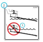
1. Do not submerge the cutter head in water.
