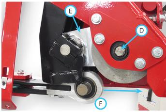
7. Pull the blade bearing housing straight back to remove the blade assembly from the cutter bar.
