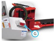
is off, the main arm pivot function is selected. When the light is on, the cutter bar pivot function is selected.
