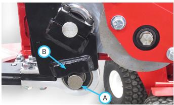
2. Position the blade assembly in the cutter bar by placing shims between the blade bar and the upper blade guides.
