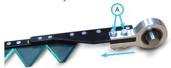
2. Install the blade bearing housing onto the new blade assembly. Slide the bearing housing up against the end of the blade bar. Make sure the bearing housing is square with the blade bar. Torque the bolts to 42 Nm (31 ft-lbs).
