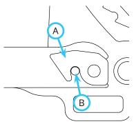
6. Raise the two jacks. Remove the ball pins and move the jacks to the operating positions. Secure with the ball pins. Secure the right jack handle with the jack handle latch.
