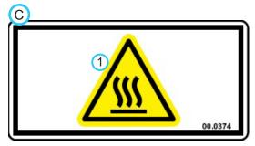
Hot surface hazard - Hot surfaces can cause severe burns. Allow engine, exhaust components, and surrounding surfaces to cool before servicing.
