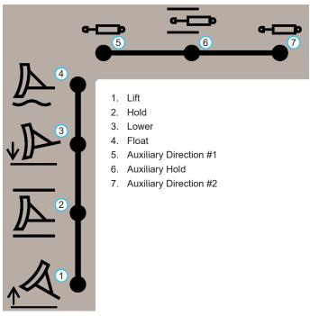
The hydraulic control lever controls the lift of the power unit's front hitch and the auxiliary hydraulic circuit.
