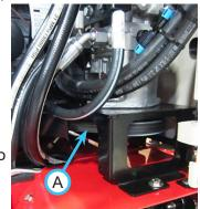
The PTO drive belt (B) can be inspected at the front hitch.
