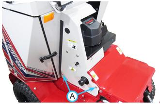
6. Install the left side cover onto the lower left engine cover mount and the accessory mount/shield frame using two 1/4 x 3/4" bolts (B) and washers. Do not tighten.
