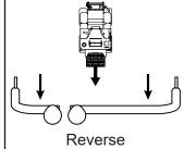
Pull the drive control levers backward to make the power unit move in the reverse direction. Changing the amount the drive control levers are moved instantly changes the ground speed of the power unit. Moving the drive control levers one half stroke will result in approximately one half of the maximum ground speed. Moving the levers to the end of the stroke will result in maximum ground speed.
