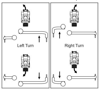
The greater the stroke variance between the left and right drive control levers, the sharper the power unit will turn.
