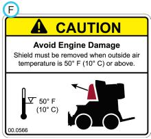
Remove the front, left, and right engine covers when the outside air temperature is 50° F (10° C) or above.
