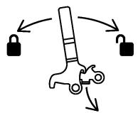
the latch tab is engaged in the attachment lower hitch plate and the latch handle lock is in place.
