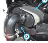
thumb screw (D) on the band clamp and remove the filter element from the intake hose.
