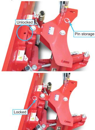
The unlocked position helps prevent sudden stops caused when contact is made with sidewalk joints, curbs, broken pavement, or other immovable objects. The unlocked position should be used for most applications. When using the plow in the unlocked position, store the pin in the hitch frame hole.
