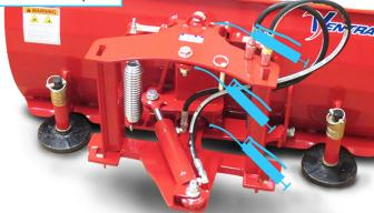
Angling the snow plow blade to the left helps increase access to the grease fitting in the lower frame pivot.
