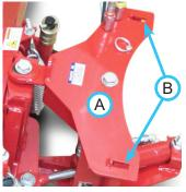
2. Drive forward slowly until the power unit hitch tabs are aligned
