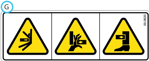
Pinching or crushing hazard.
