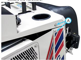
6. Install the left rear windscreen mount assembly (flange and latch are positioned toward the back of the power unit) using two 1/4 x 3/4" bolts, flat washers, and flange nuts. Do not tighten.
