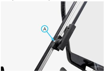
2. Install new wiper blade and reinstall the screw and nut.
