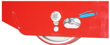
2. Grease the caster wheel axles and pivots.
