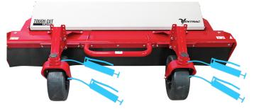
3. Grease the drive shaft bearings.
