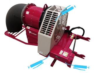
2. Grease the wheel axle bearing and the caster wheel pivot.
