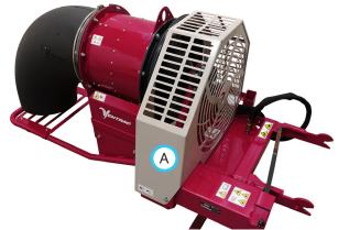
3. Release the turbine fan belt tension spring.
