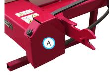
4. Reinstall the drive pulley shield.
