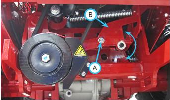
3. Tighten the adjustment bolt securely. Torque to 42 Nm (31 ft-lbs).
