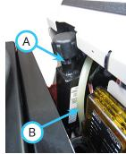
6. If the hydraulic oil level is below the low mark on the decal, add HydroTorq XL synthetic hydraulic oil until the proper level is reached.
