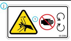
1. Cutting or pinching hazard. Stay away from moving parts.
