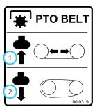
Pulling the PTO belt tensioner rod out (2) releases the belt tension, allowing the operator to remove or install the attachment drive belt.
