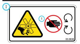
1. Severing of fingers or hand - engine fan. Stay away from moving parts.
