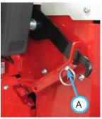
Ensure the shift lever is secured in the lock position at the end of the shift stroke. Reinstall the
