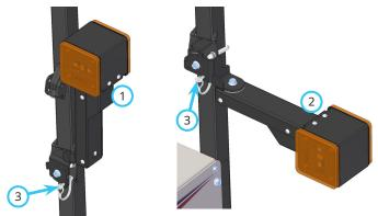
To change the light position, remove the lock pin (3), move the arm to the desired position, and reinstall the lock pin to secure in place.
