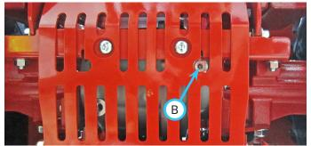
Remove the drain plug (B) from the rear transaxle and allow the hydraulic oil to drain. Remove the oil fill plug (C) from the rear transaxle to allow venting. NOTE: on some
