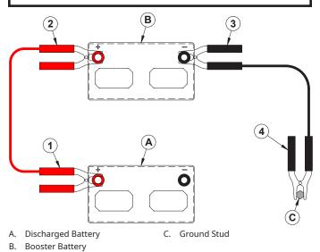
5. Connect one end of the positive (+) booster cable to the positive (+) terminal (1) of the discharged battery.
