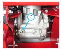
power units, it may be necessary to remove the rear transaxle skid plate to access the drain plug.
