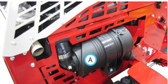
2. Release both latches (B) on the engine air filter assembly (A) and unhook the latches from the main filter housing.
