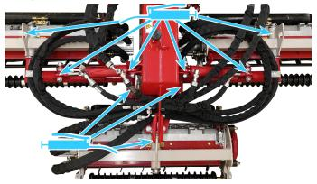
Grease the rear roller bearings (6 places), the front roller bearings (6 places), and the motor shaft (3 places). Grease the motor shaft until excess grease comes out the grease vent at the top of the motor side plate.
