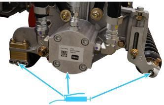
If equipped with an optional brush kit, grease the brush shaft bearings (6 places).
