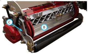
To open the rear shield, loosen the bolt (C) securing the shield to the left side plate, rotate the shield to the open position, and tighten the bolt.
