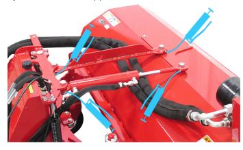
Brush Rotor Bearings (2), Wheel axles (2), and Caster Pivots (2)
