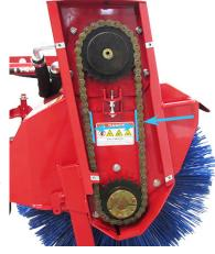
correct, reinstall the drive chain cover and torque the bolts to 8 Nm (67 in-lbs).
