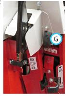
Pull the secondary SDLA lever to the left to tilt the bucket or tool back toward the power unit. Push the secondary SDLA lever to the right, to dump the bucket or tilt the bucket or tool forward away from the power unit.
