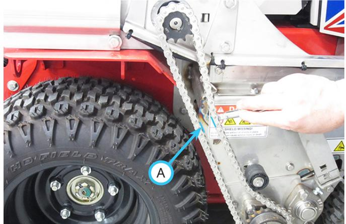
NOTE: measure the distance (A) between the two chain strands with and without pressure applied to determine the amount of chain deflection.
