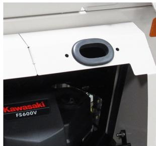
41. **2100:** Route the controller power cord through the grommet in the engine cover.
