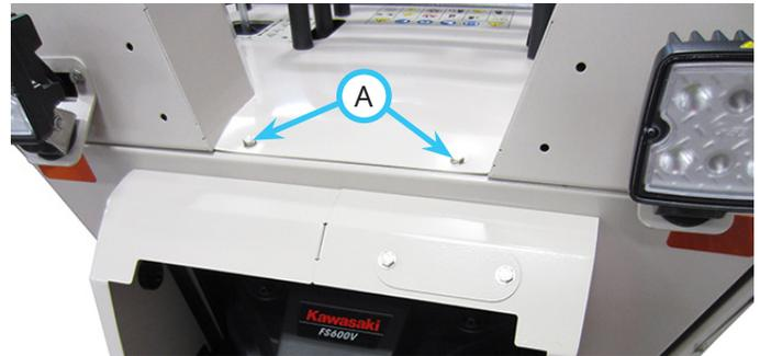
3. Power units with serial numbers 01001 - 01230 will require mounting holes to be drilled in the outer dash panels. For power units outside of this range, skip to step 8.
