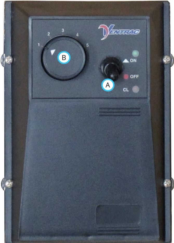
Rotate the dial to select the desired speed setting. Position #1 is the minimum speed setting and position #5 is the maximum speed setting.
