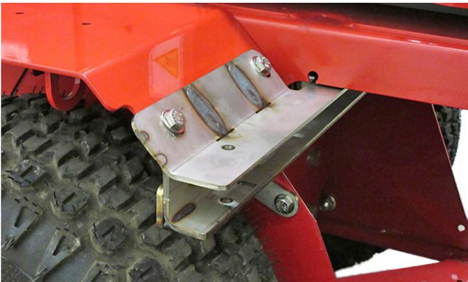
13. Install two 5/16 x 3/4 inch bolts (D) and washers through both the left and right side flanges and secure with flange nuts.
