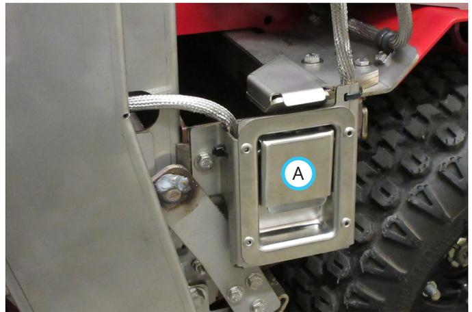
The hopper latch secures the hopper in the power unit during operation. Lift up on the latch handle (A) to disengage the latch so you can slide the hopper out of the power unit when filling the hopper with material. When sliding the hopper back into the power unit, check to make sure the latch is engaged before returning to operation.
