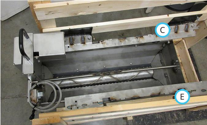
12. Secure the roller rail to the front fenders using the hardware from the crate. Do not tighten the hardware.
